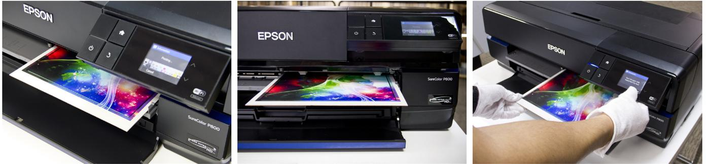
Once it's finished printing, push the eject on the P800's control panel, then select 'yes' to unload the panel.
