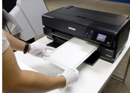
Always make sure the Platen Gap/Head Height setting on your printer is set to the highest/widest possible setting.
